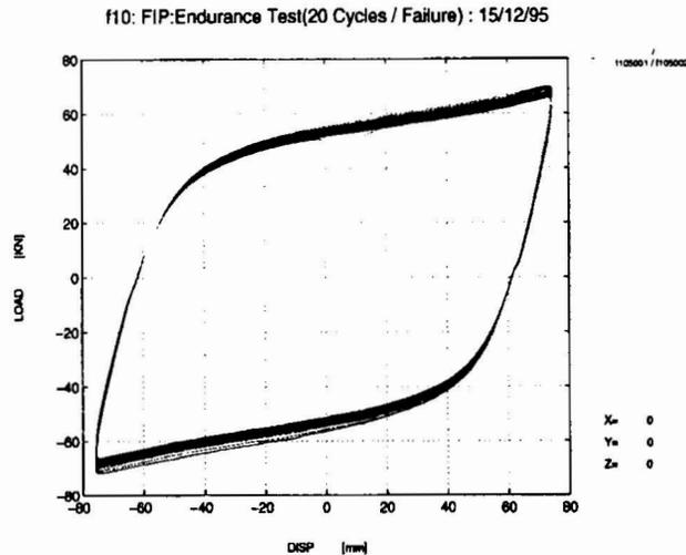
Figure 5: Hysteretic Energy Loss of Steel Dampers used on Granville Bridge
