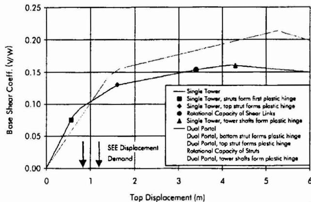
Figure 8: East Bay Bridge - Lateral Load Response of Single Tower and Dual towers of Suspension Bridge
