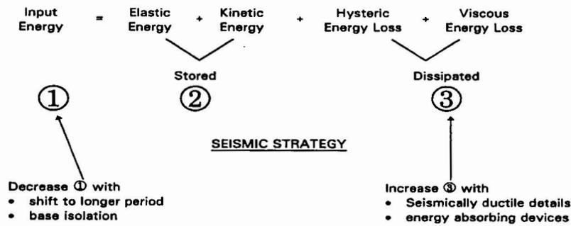
Figure 4: Seismic Energy Balance for a Bridge Structure
