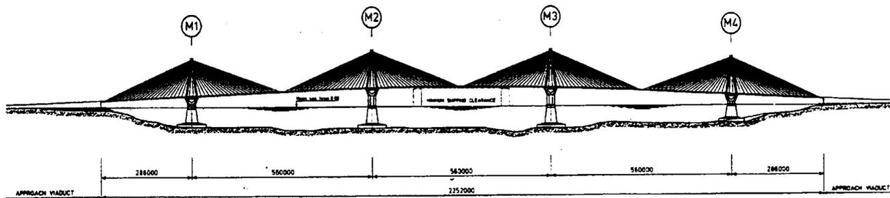
Figure 9: Elevation Rion Antirion Bridge, Greece
