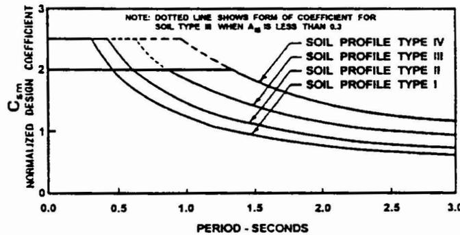
Figure 2 - Normalized Seismic Response Coefficients for Various Soil Profiles in AASHTO LRFD
